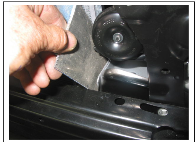
Figure 10 – Steel backstop (supplied).
